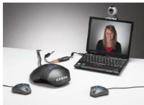
Pic 4: Konftel 60W with/without microphones connected to Alcatel IP Softphone via cable/USB or Bluetooth.
